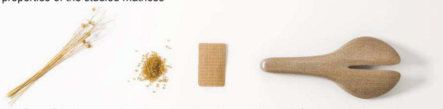
Fig. 3 From flax plants and cellulose based polymers to natural fibre composite parts
